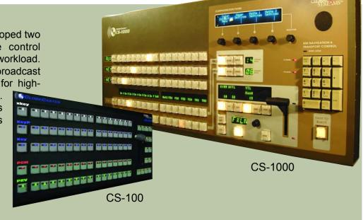
Because of GlobeCaster's modular architecture, every system is built with the inputs and outputs our customers specify. Changing formats? Just change cards.
