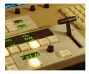
Though GlobeCaster is many tools in one device, video professionals can spread the workload using the optional switcher control surfaces, CS-1000 and CS-100. These separate components allow one person to control the video switching while another prepares and loads graphics. However, even with this panel GlobeCaster remains one complete tool.
