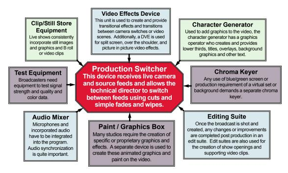
A different manufacturer makes each of these various pieces of broadcast equipment, and each requires significant capital investment - from \$200,000 to \$millions. Also, each piece of equipment requires an experienced operator. Each device and manufacturer has its own training requirement, support organization, and warranty program. Operating and managing this collection of equipment requires significant monthly expense.
