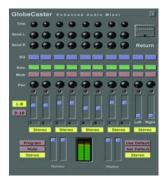
GlobeCaster also allows you to mix up to 16 channels of audio. Of them are 8 channels of balanced XLR production audio as well as 8 virtual channels of audio used for DV and DDR playback inside GlobeCaster. This mixer application provides the ability to adjust high, mid and low bands with a powerful three-band parametric equalizer.
