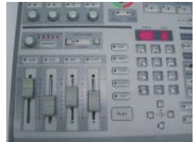
Four channel Audio mixer with A/V sync calibration
